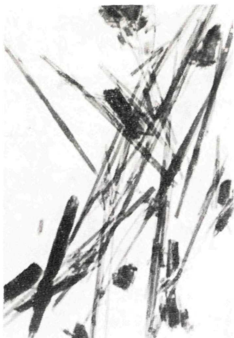
Fig. 20. Prevalence of fibrous chrysotile over lathes (lizardite—brucite—antigorite ?); sample 4a, Jaklovce. Magnif. 7000 \times , TEM
