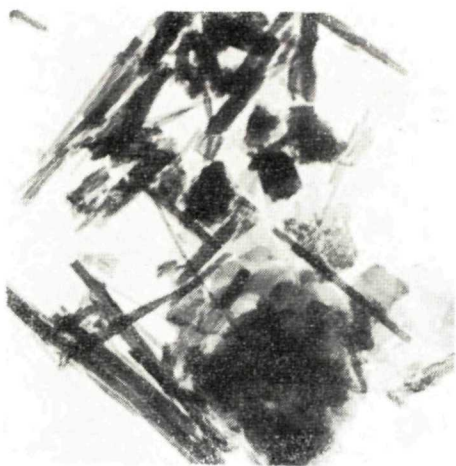
Fig. 22. "Deweylite" (= mixture of chrysotile and isometric tabular lizardite). Sedlice. Magnif. 7000 \times , TEM Obr. 22. „Deweylit“ (= zmes chryzotilu a izometricko-tabuľkovitého lizarditu). Sedlice. Zväčš. 7000 \times , TEM
